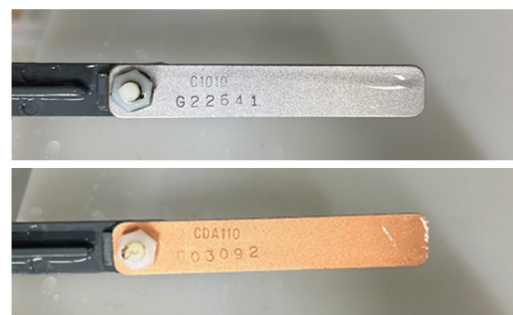
Coupons from corrosion study after treatment with EcoSHIELD
